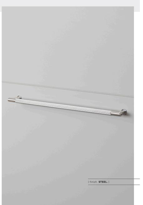
[ type. **HARDWARE.** ] [ info. MEASUREMENTS.] 15 mm 12 mm 5/8" 4/8" 350 mm 325 mm 13<sup>6</sup>/8" 12<sup>6</sup>/8" [ info. **SPECIFICATIONS.**] 1 pull bar with 2 small discs Rear fixing Fits doors of: Max 20mm or 25/32"\* 36 mm 13/8" \*For thicker doors you will need to source longer M5 screws
