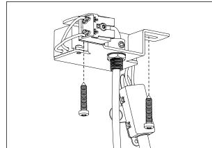
Mount the bracket to the ceiling with screws.
