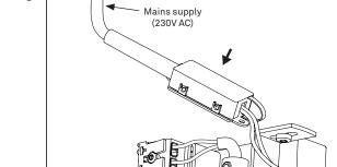
CAUTION: Connecting mains supply 230V AC directly to the pendant will damage the LED-module.
