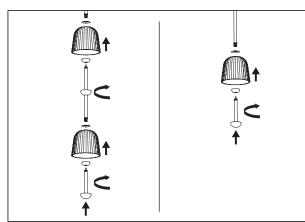
Lead the curved washer through the thread.
