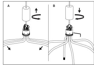
**A:** Unscrew and remove the cover carefully.
