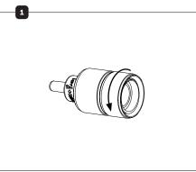
Unscrew the smaller metal ring from the light fitting.
