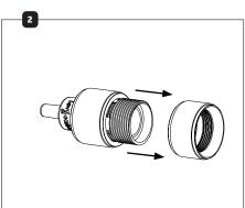
Feed light fitting through hole in the bottom of the bar. Re-attach metal ring back onto the light fitting, through the metal cage. Fix light bulb into light fitting.
