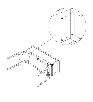
**5** Ensuring the screws are properly installed, carefully stand the rockstar upright.
