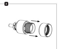
Feed light fitting through hole in the side of the bar. Re-attach metal ring back onto the light fitting, through the metal cage.
