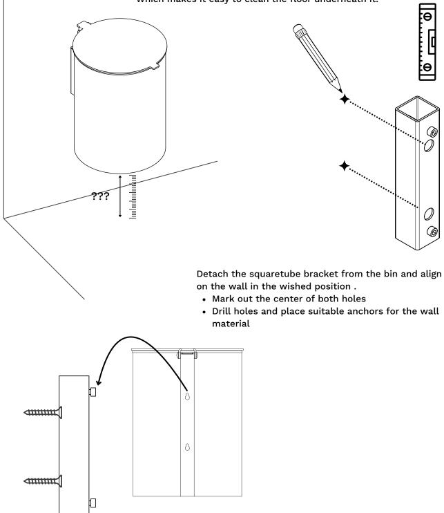
When mounted on the wall, leave the M4 bolts no more than 2mm from surface to slide down the bin through the key-slots. If the bin seems jiggly, try tighten the screws 1 round more.
